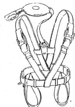
A Full Safety harness with fall arrest block
